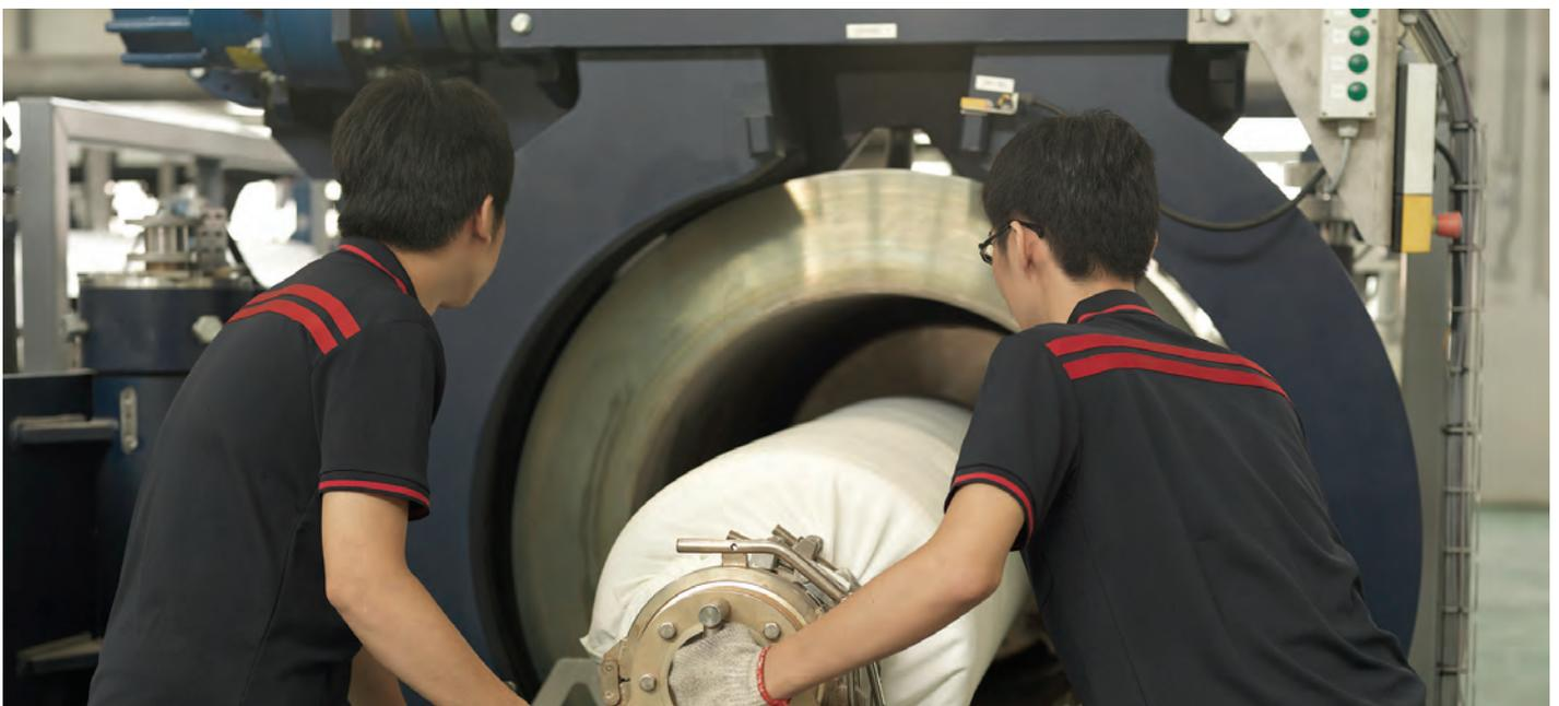
Loading fabric into the vessel
